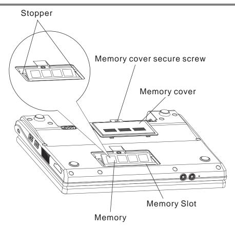
Figure 4-3 Removing the optional memory
